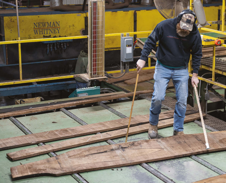
Left: Inspector Sean New flips boards so he can examine and mark them for the 11 different grades of lumber. Properly grading lumber can make or break the company. These skills are learned at schools put on by the National Hardwood Lumber Association, which set standards for lumber grading not long after its establishment in 1898. Right: Nothing is wasted at MO PAC Lumber. Sawdust and scrap pieces of wood are burned to create steam and to heat the drying kilns. What's left is sold to a company in Auxvasse that turns them into landscape mulch, or they go to the University of Missouri where they help fuel its power plant.
