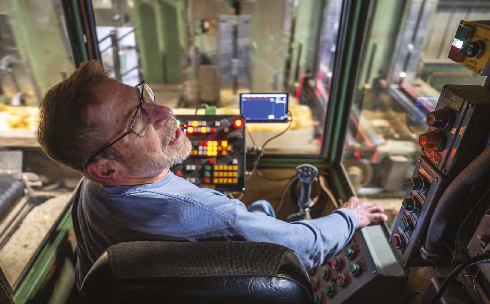
Above: Scott Schrader is one of the most experienced among the highly skilled workers at MO PAC Lumber. He has spent 43 years behind the controls of the bandsaw that turns logs into lumber. He works two joysticks with seven buttons each to override the computer programming and manipulate logs for the best cuts. Below: Freshly cut lumber is sorted by thickness and stacked on carts so material handlers Matt Overstreet, left, and Gauge Weaver can wheel them to an all-concrete building where the boards will be steamed for 84 hours to ensure uniform color. Right: Rakiim Chairse-McCutcheon loads steamed and dried boards onto rollers where they will move to be graded, a critical step in adding value to the wood.
