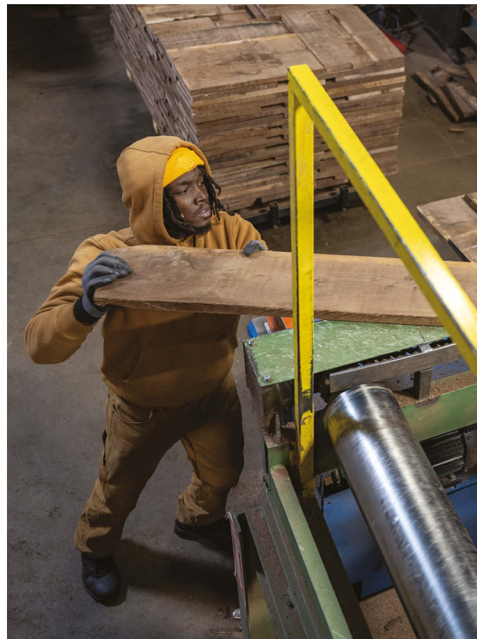
Above: Scott Schrader is one of the most experienced among the highly skilled workers at MO PAC Lumber. He has spent 43 years behind the controls of the bandsaw that turns logs into lumber. He works two joysticks with seven buttons each to override the computer programming and manipulate logs for the best cuts. Below: Freshly cut lumber is sorted by thickness and stacked on carts so material handlers Matt Overstreet, left, and Gauge Weaver can wheel them to an all-concrete building where the boards will be steamed for 84 hours to ensure uniform color. Right: Rakiim Chairse-McCutcheon loads steamed and dried boards onto rollers where they will move to be graded, a critical step in adding value to the wood.
